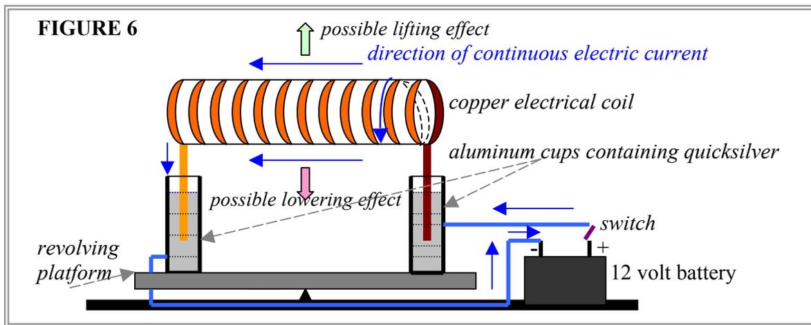
The draft above illustrates the basic concept that promoted the test. The rigid extremities of the electrical coil are immersed in quicksilver and tend to float. The aluminum cups are well connected to the electrical circuit.
